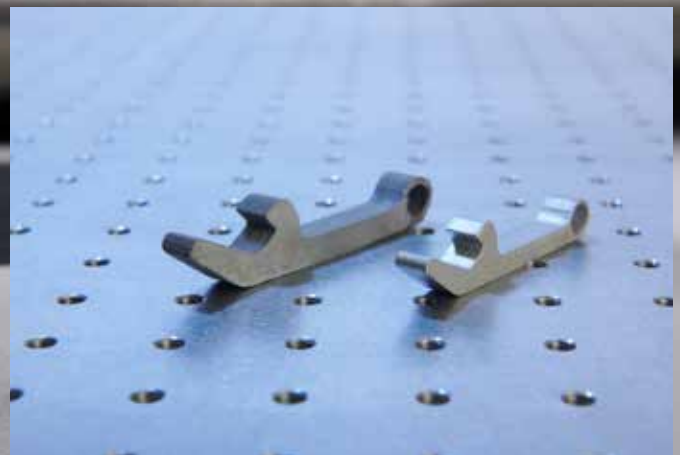
Binder jetting (left: green body, right: finished component)
